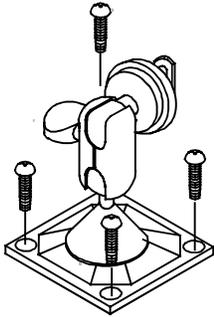
**3** Assemble the display to the bracket by aligning the "T" in the slot and hand tightening the nut and lock nut.
